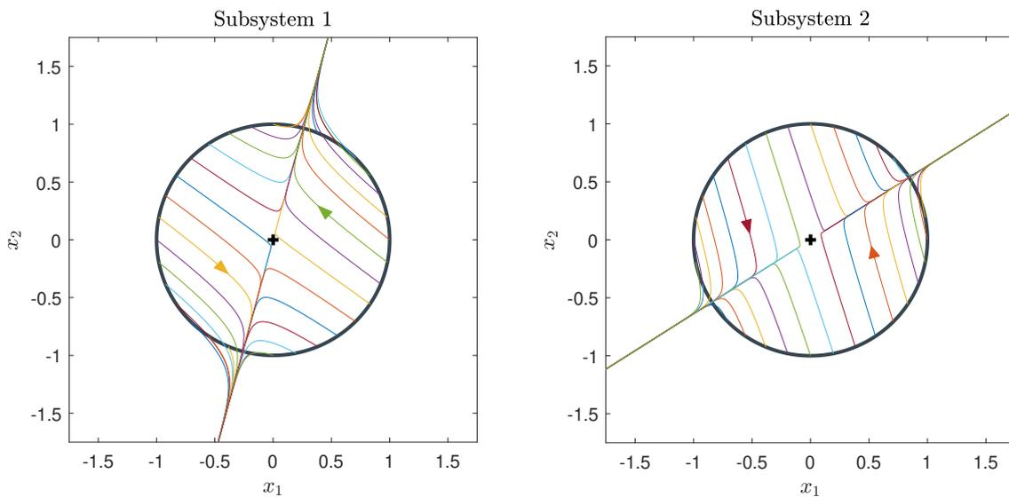
Figure 3.2: Phase portrait for each unforced linear subsystem.
