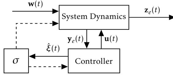
Figure 4.1: Closed-loop system.
