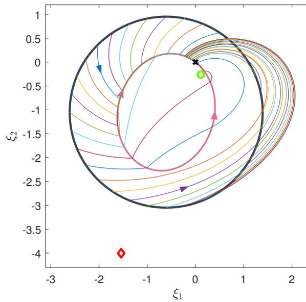
Figure 3.6: Phase portrait for the switched affine system under the min-type quadratic rule.
