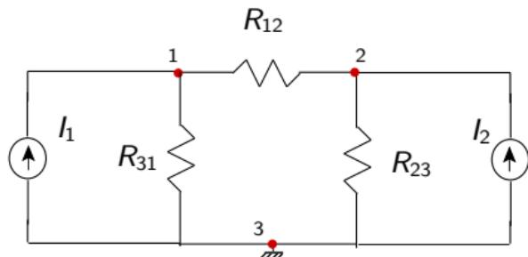
$$\begin{bmatrix} \frac{1}{R_{12}} + \frac{1}{R_{31}} & -\frac{1}{R_{12}} \\ -\frac{1}{R_{12}} & \frac{1}{R_{12}} + \frac{1}{R_{23}} \end{bmatrix} \begin{bmatrix} E_{13} \\ E_{23} \end{bmatrix} = \begin{bmatrix} I_1 \\ I_2 \end{bmatrix}$$
