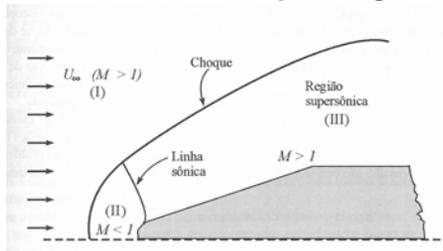
$$\frac{\partial^2 \phi}{\partial x^2} - \frac{1}{(M^2 - 1)} \frac{\partial^2 \phi}{\partial y^2} = 0$$
