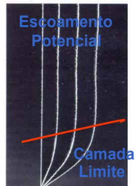
Fig. 21. Velocity profile in the laminar bound dary layer (0.01% salt water, free stream velocity 0.6 cm/s, distance from the leading edge 200 mm,  $Re = 1.2 \times 10^5$ , hydrogen bubble method).
