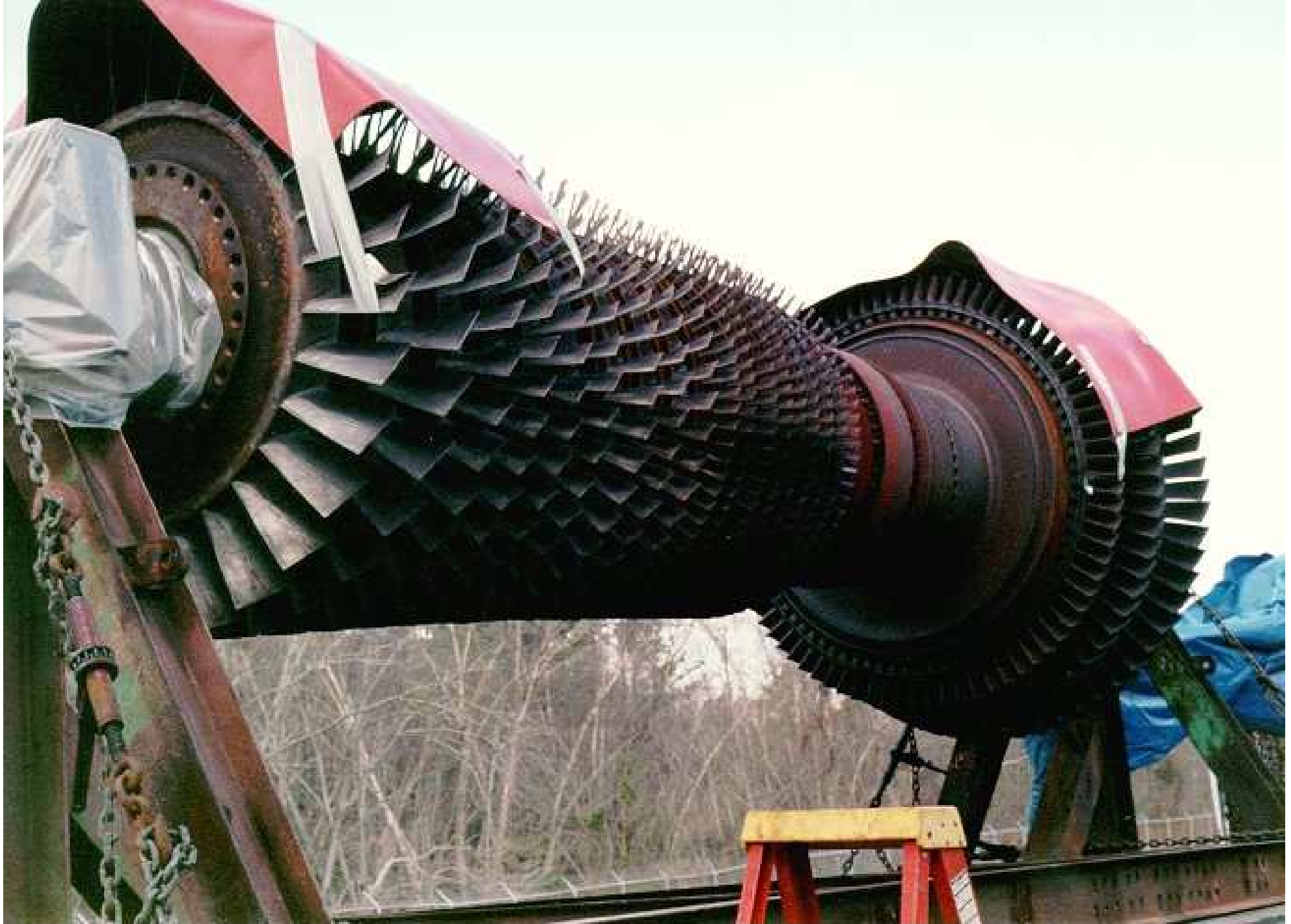
Compressor and turbine rotor blades for an industrial gas turbine. (Courtesy of S. Laney)
